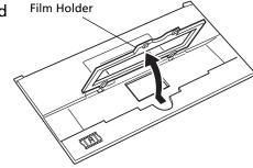
**3** Place the film face down into the groove in the Film Guide.
